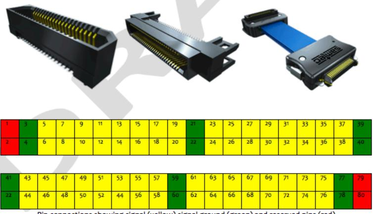
Pin connections showing signal (yellow) signal ground (green) and reserved pins (red)
