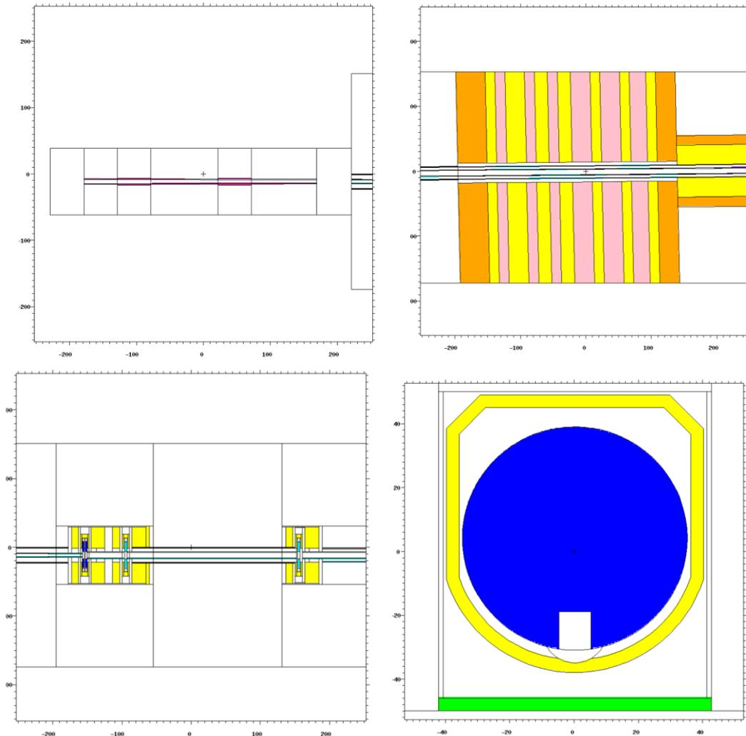
Fig. 1: (above) Geometry of the NBOA and bunker-wall feedthrough; (below) Geometry of the choppers (1 to 4).
