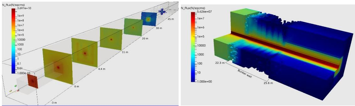
Fig. 3: Neutron flux at several distances along the X axis( left) in the bunker and (right) at the bunker wall.
