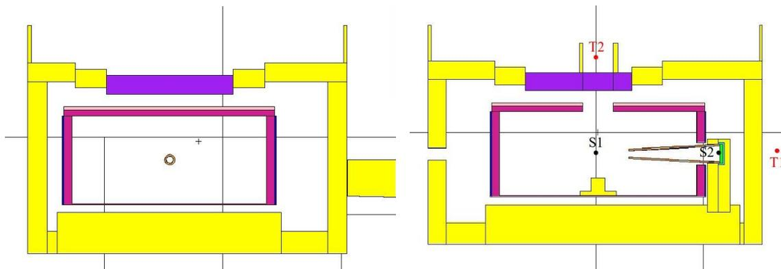
Fig. 6: (left) YZ cut view, and (right) XZ cut view of the MIRACLES cave. S1 (sample) and S2 (B<sub>4</sub>C canister) are the gamma sources under study.
