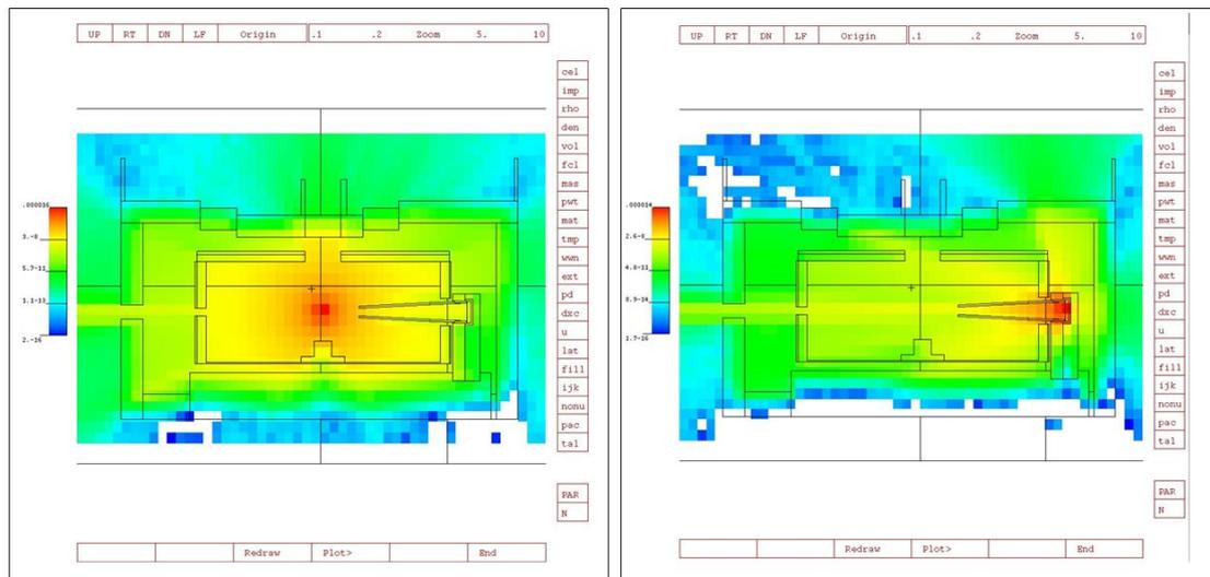
Fig. 7: Dose distribution inside and outside the experimental cave splitting two main gamma sources: (left) sample source, S1 and (right) beam stop source, S2.
