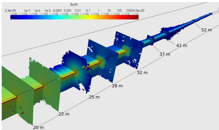
Fig. 4: Neutron dose rate, overall view along the X axis.
