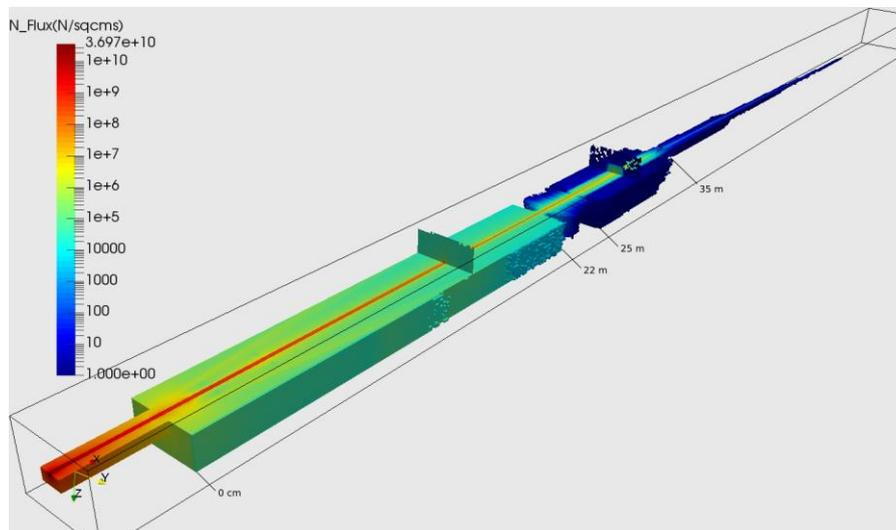
Fig. 2: Neutron flux, overall view, cut at  $Y=10$  cm and 2 slides, 1st slide in-bunker 2nd slide ex-bunker
