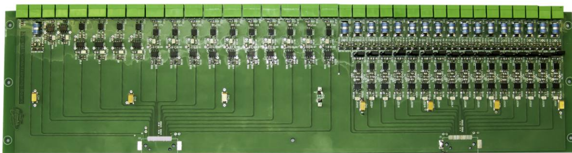
Figure 17 Assembled PCB of Digital Conditioning Board.
