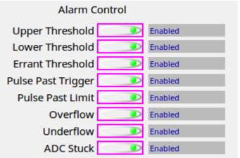
Alarm status is available for monitoring purposes as well as for MPS interfacing
