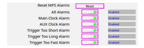
Alarm status is available for monitoring purposes as well as for MPS interfacing
