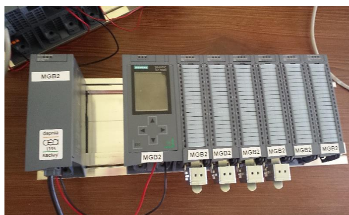
Figure 26: PLC system for the gas control example, with the CPU and Siemens cards connected.
