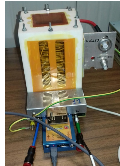
Quad-Timepix2 Timepix 2: 256 \times 256 pixels with dimension 55 \times 55 \mu\text{m}^2
