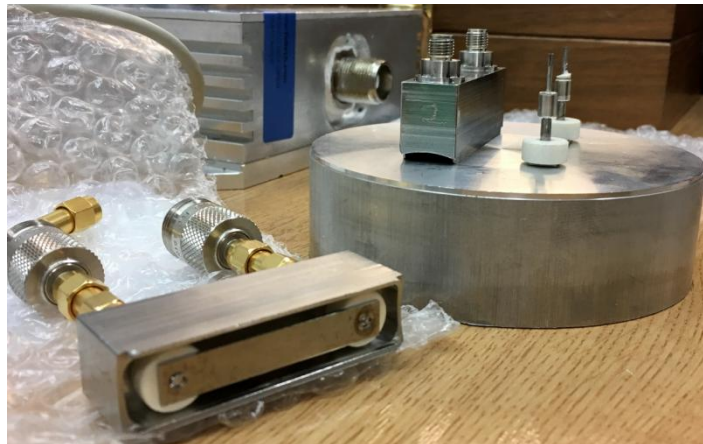
Figure 3: SL-Box welded and ready for checks during prototype process.
