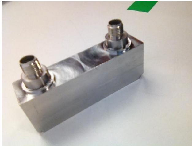
Figure 1: Two feedthroughs e-beam welded to SL-Box during prototype process.
