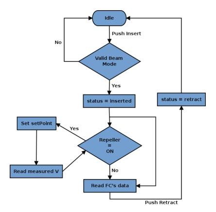
From the flow diagram we observe that from the idle position the operator decides to insert the FC. The IOC will check the Beam Mode status and depending of this status will continue to block the user in the idle position or will allow the setting of the repeller. The use of the repeller will be optional.
