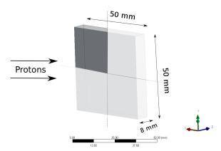
The straight plate is the model simulated because it is the worst case for the BS in nominal conditions. This allows to normalize the limits and adapt them to other geometries with different footprints.
