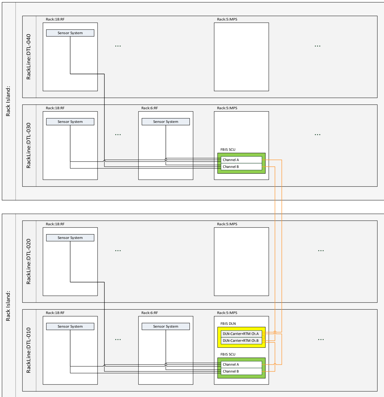
Figure 30: Similar sketch to Figure 28 but the redundant channels of the SCU, DLN and SLink are explicitly shown.
