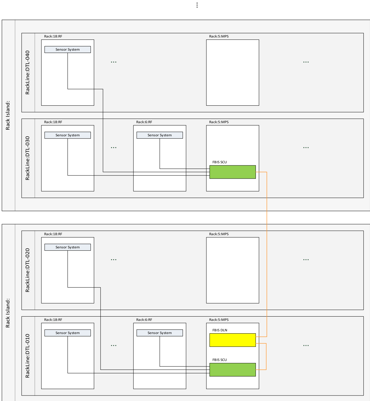
Figure 28: Deployment of a DLN and SCUs along the Klystron Gallery. The orange lines represent SLink interfaces.
