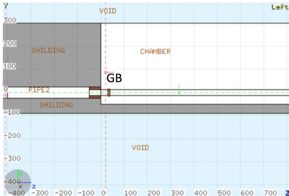
Figure: 12 Beam Dump section geometry in FLUKA
