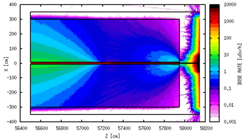
Figure 6 : Residual dose rate after 5 years of exposure and no cooling times
