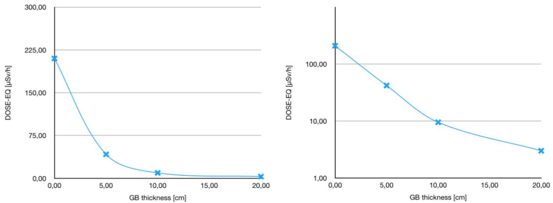
Figure 15 : Residual dose rate after 5 years of exposure at various cooling times inside the 'beam pipe' as a function of GB thickness
