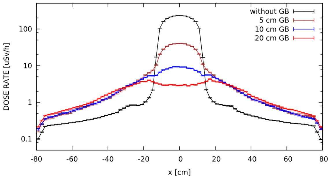
The level of the dose rate was calculated on a cross section of the dump tunnel. The location of this measurement is on the GB contact plane behind the GB, see Figure 15.
