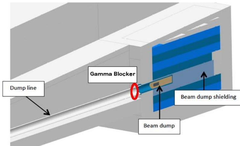
Figure 5 : Location of gamma blocker in dump line region
