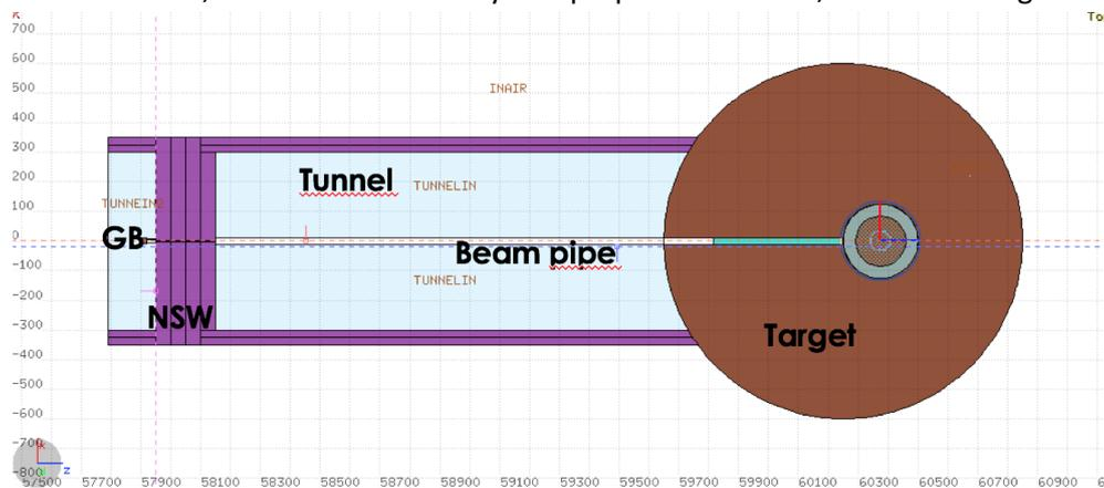
Figure 4 : Target Geometry in FLUKA
