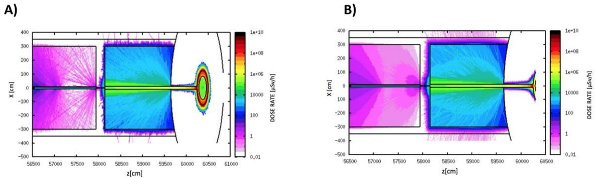
Figure 2: The residual dose rate in the last 40 m of A2T, with NSW and Target Wheel
