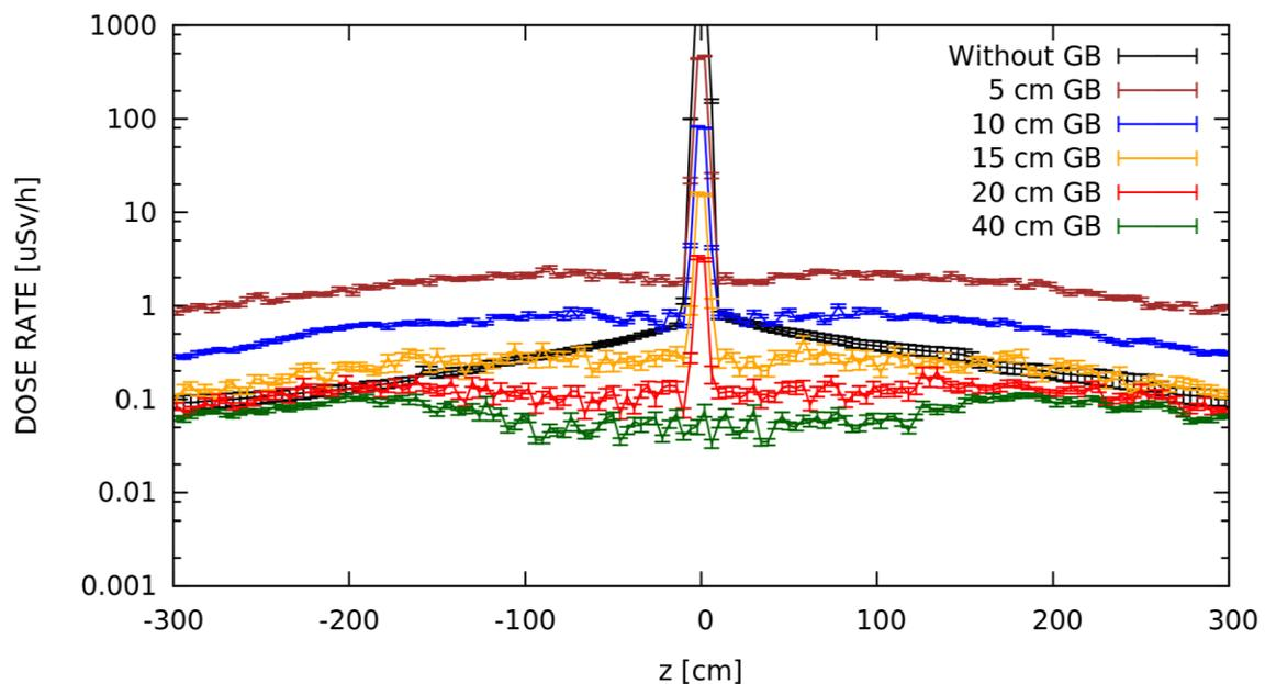
Figure 10: Residual dose rate vs. distance from the beam pipe. Projection on X-axis. Z=57400cm. 5 years of exposure, cooling time 0s, GB thickness: 0cm, 5cm 10cm,15cm 20cm 40cm GB
