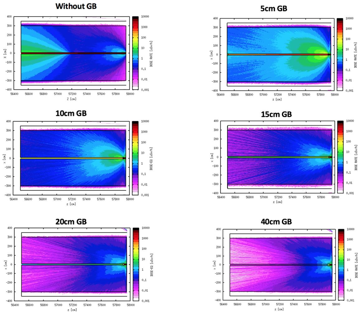
Figure 8 : Dose rate after 5 years of exposure, no cooling time for different steel GB thicknesses
