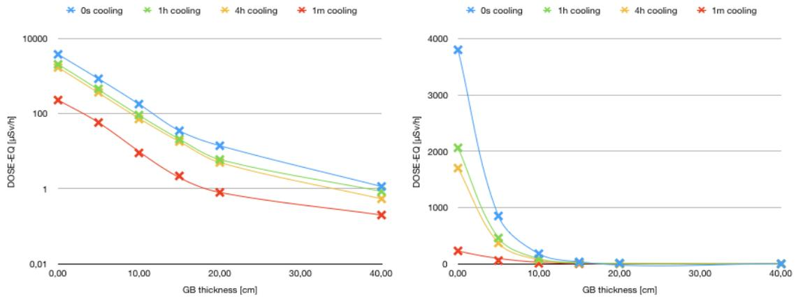
Figure 12 : Residual dose rate after 5 years of exposure at various cooling times inside the 'beam pipe' as a function of GB thickness
