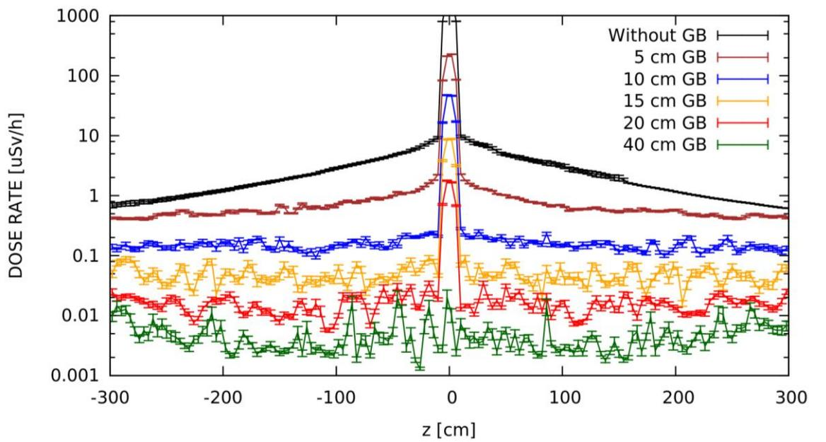
Figure 11 : Residual dose rate vs. distance from the beam pipe. Projection on X-axis. Z=56500cm. 5 years of exposure, cooling time 0s, GB thickness: 0cm, 5cm 10cm,15cm 20cm 40cm GB
