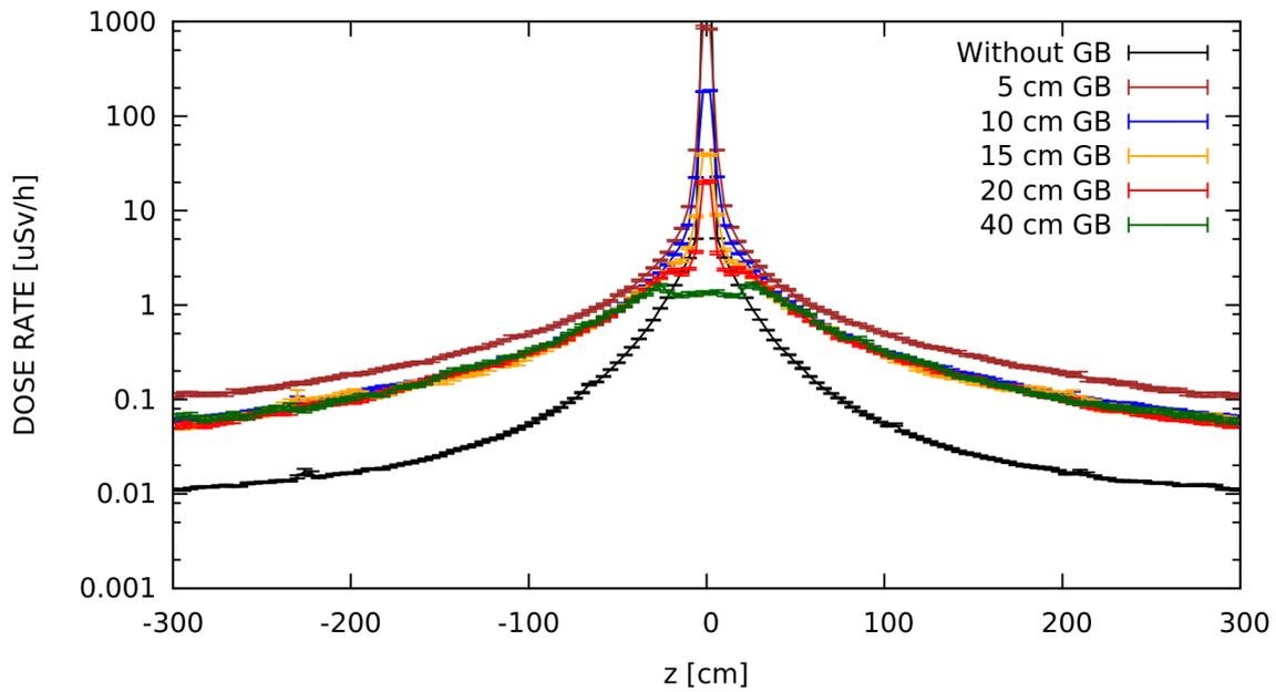
Figure 9 : Residual dose rate vs. distance from the beam pipe. Projection on X-axis. Z = on GB contact (on the NSW contact in situation without GB). 5 years of exposure, cooling time 0s, GB thickness: 0cm, 5cm, 10cm, 15cm, 20cm, 40cm
