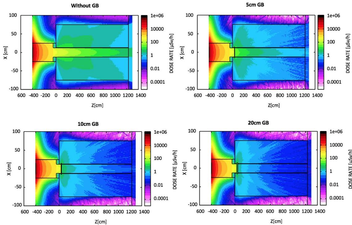
Figure 13 : Dose rate after 50 years of exposure, no cooling time, without GB for different steel GB thicknesses
