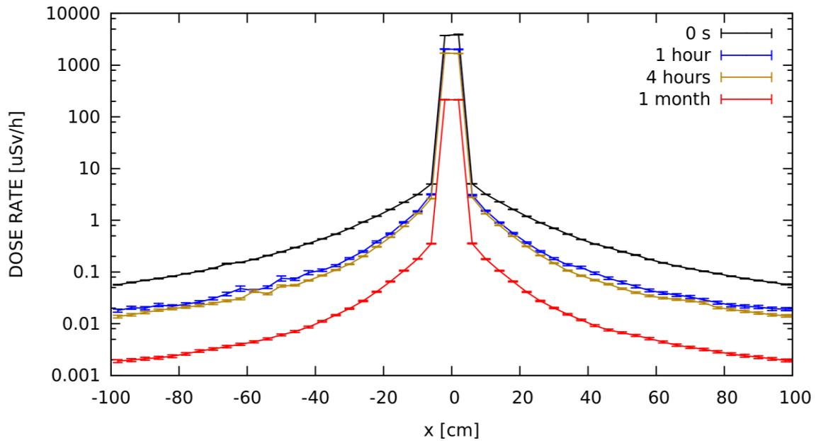
Figure 7 : Gamma radiation dose rate vs. distance from the beam pipe. Projection on X-axis. Cooling times: 0s, 1hour, 4 hours,1 month (black). Z=57950cm
