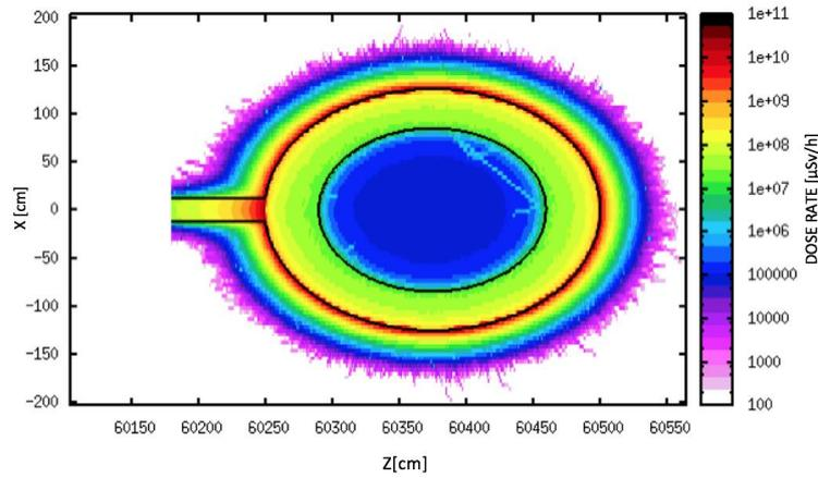
Figure 1: Implemented isotropic source on the external target wheel surface
