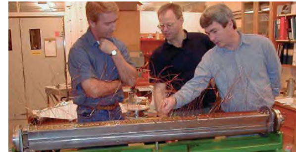
Old MAX-Lab wiggler with 3.5T peak field at 4K
