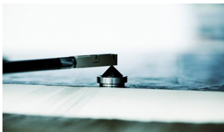
Alignment with magnet tip within 10 \mu\text{m}
