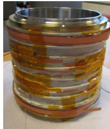
Coil with 8 sub-coils
