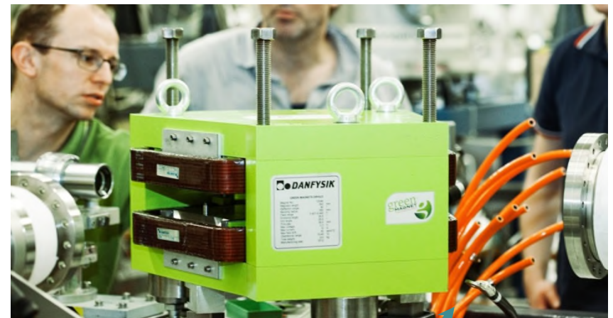
Water hoses and thick power cable needed for the original conventional electromagnet
