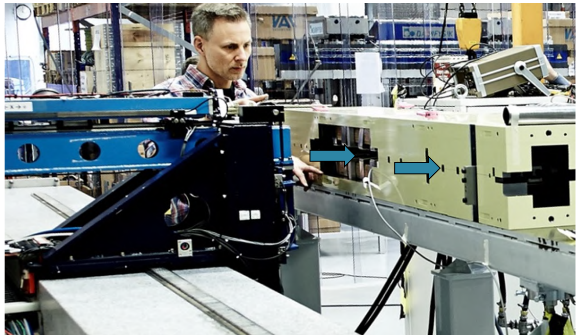
Scanning dipole from side & quadrupoles through small holes in yoke
