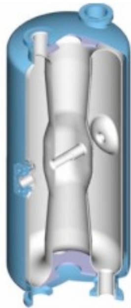
HWR, 172.5 MHz, \beta_{\text{opt}}=0.25 Half wave resonator
