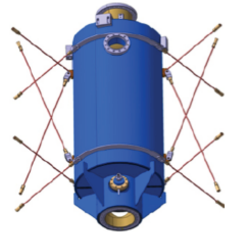
Figure 4.120: Helium vessel with hanging rod
