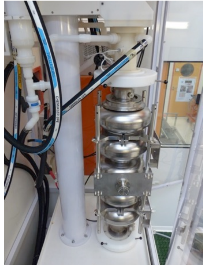
Vertical Electropolishing system@ CEA
