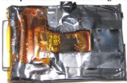
Fig 2: Timepix3 detector with 5um B 4 C coating with about 80% 10 B.
