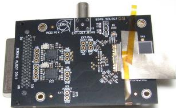
Timepix3 detector with 25um gadolinium foil.
