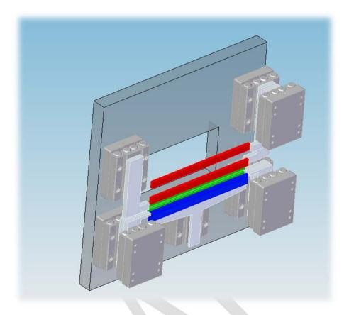
The horizontal blades and back plate have been removed in this view
