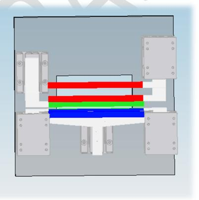
This is an initial concept of the small set of slit that is closest to the sample. The space envelope this would take up would be between. 100mm (h) x 100mm (w) x 50mm (t) minimum size and a maximum size of 200mm (h) x 200mm (w) x 100mm (t)
