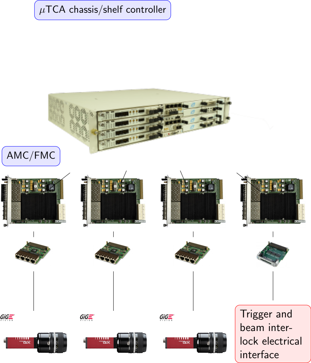
Figure 1: Image capture and processing hardware overview. Can we still use this? Probably at least change to selected HW
