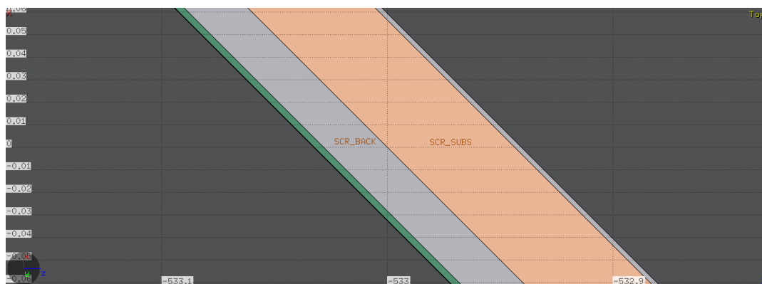
Figure 5 Details of layers for structure of simulated screen. Coating = GREEN, Backing = GREY, Substrate = PINK, Mirror = GREY. Total thickness = 650 \mu\text{m}
