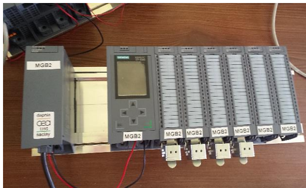
Figure 5: PLC system for the gas control, with the CPU and some analogic and digital Siemens cards used.
