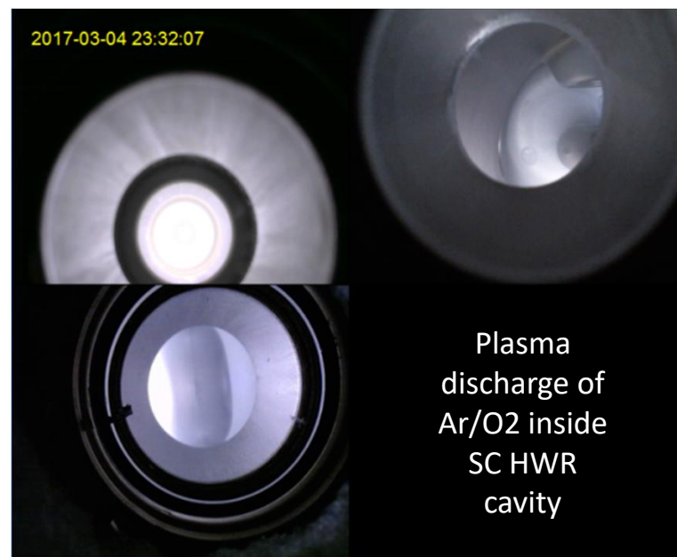
Fig. Plasma cleaning setup for HWR (left) and picture of discharge on the cavity (right)
