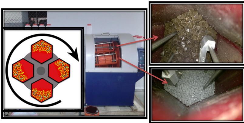
Centrifugal Barrel Polishing machine with oblique axis
