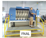
Mass Finishing for 0.65 and 1.3GHz
